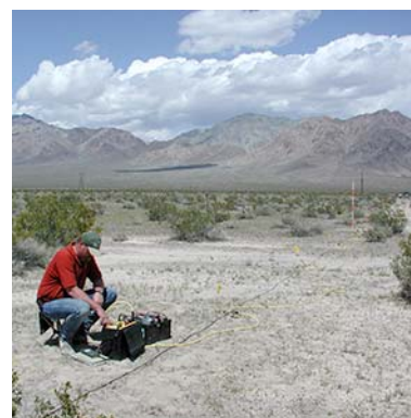
Fig. 4. DC resistivity measurements.
